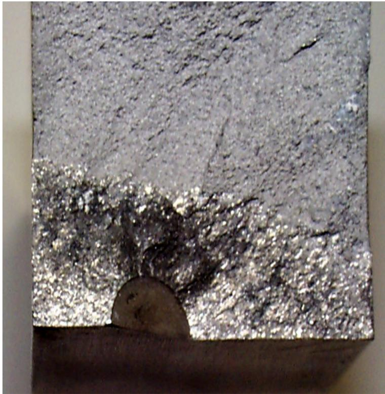
Figure 20. Final observed crack shape. The shiny fracture surface is the fatigue crack; the duller surface is a fast fracture.
